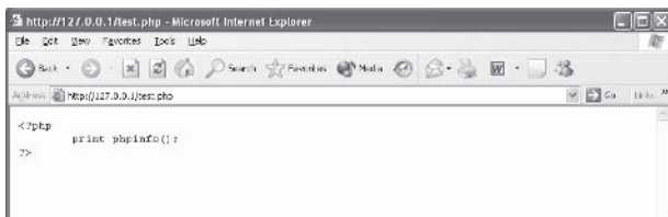
Figure 3-8 A failed PHP installation
